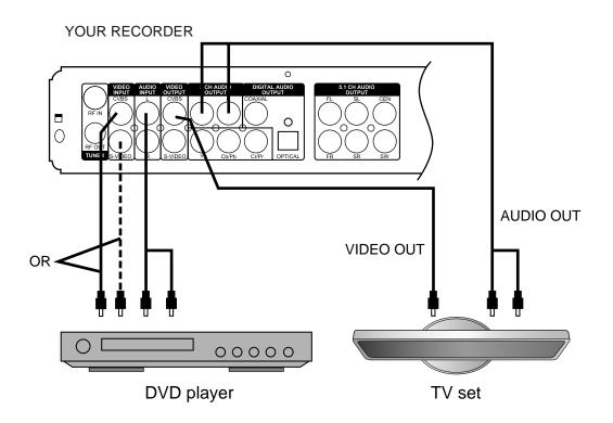
Connect your recorder with the S-Video cable, if the Signal Source has an S-Video input. Do not connect the yellow video cable if using the S-Video cable.
